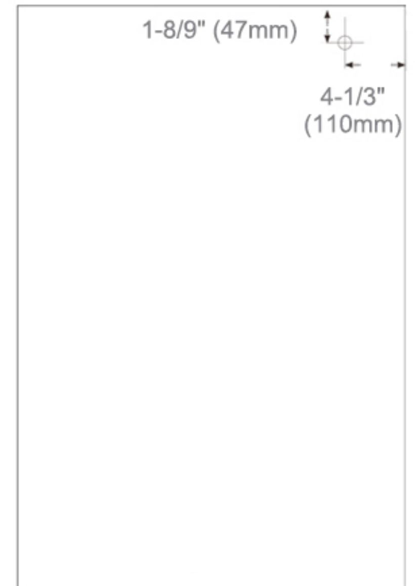
Back of Cabinet - Wire Access Location
