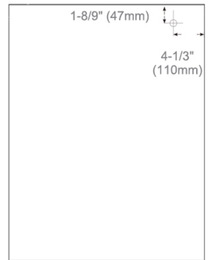
Back of Cabinet - Wire Access Location
