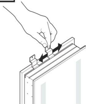
Make sure top brackets are locked in the grooves.
