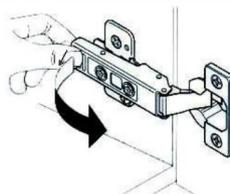
To secure hinge to mounting plate:
