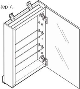
Connect the glass shelves (C) to the cabinet by pushing the side of the shelf in the left or right clip and snapping the shelf down.
