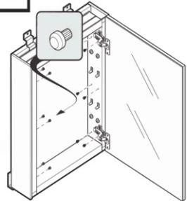
Insert clear plugs into the remaining/unused holes of the cabinet.
