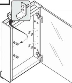
Insert clear snap in shelf clips into holes on the sides of the cabinet.
