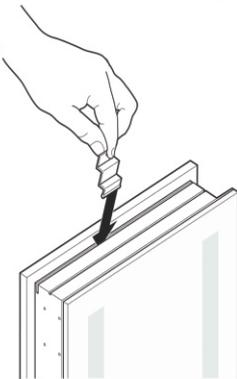
Slide top brackets into channel at the top of the cabinet.
