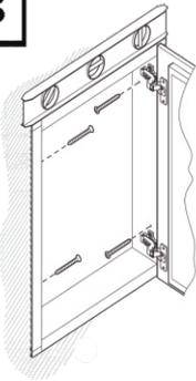
Level, then secure the medicine cabinet with the screws through the mounting holes into the framing studs.
