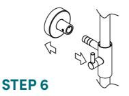
Remove the riser and the mounting piece.
