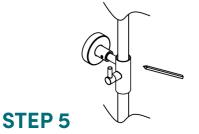
Makesure the riser is level, mark the position of the screw holes.
